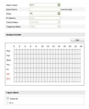
Figure 6-31 Alarm Output Settings
