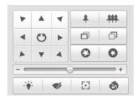
Figure 5-2 PTZ Control Panel
