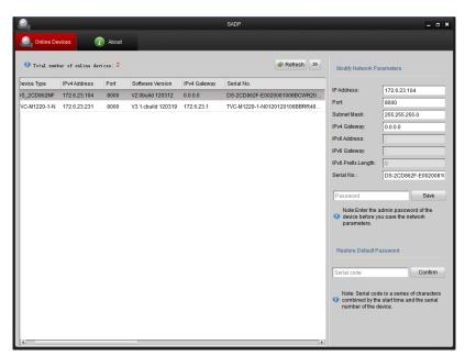
Figure A.1.2 Modify Network Parameters
