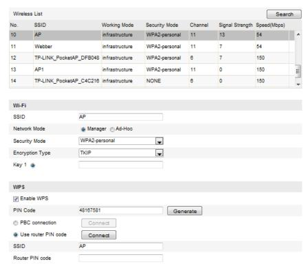
Figure 4-8 Wi-Fi Settings – WPS PIN Mode
